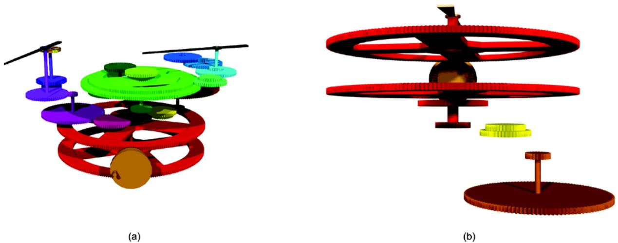
Figure 4: Two frames from the original animations. (a) A frame showing the differential gear at the top. (b) A frame showing the assembly of the mechanism by the gears falling into place.
