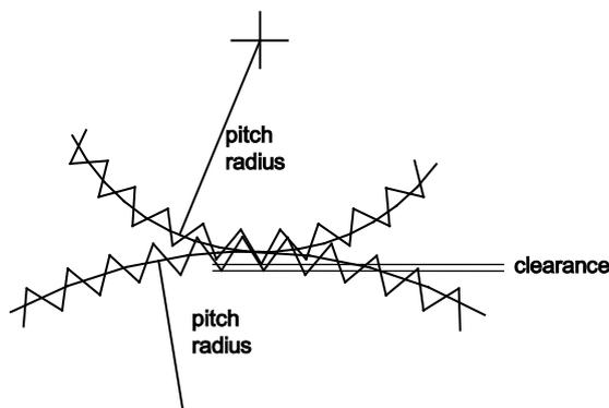
Figure 6: Gear parameters.
