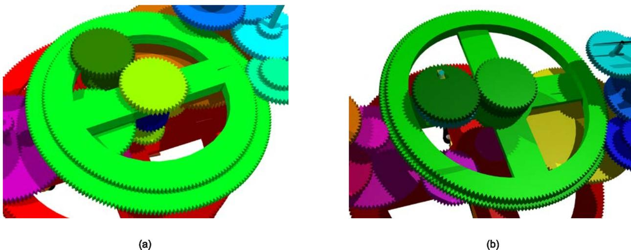
Figure 7: Replacement of the differential gear. (a) Price's differential gear (b) Hipparchos' gears in the new model.
