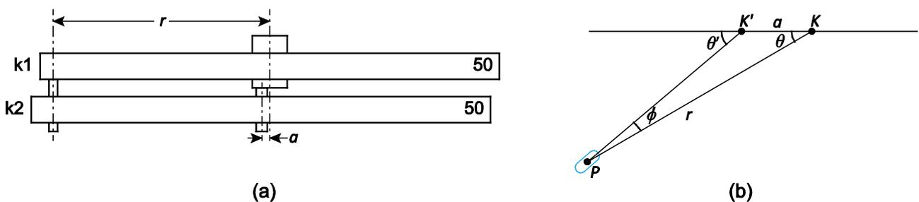
Figure 5: Calculation of the relative angle of the slotted Hipparchos gear.
